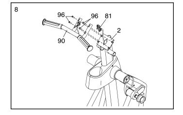
While a second person holds the Console (3) near the Upright (2), connect the three wires on the console to the Upper Wire Harness (81), to the Pulse Wire (92), and to the Ground Wire (97). Insert the excess wire into the Upright.
